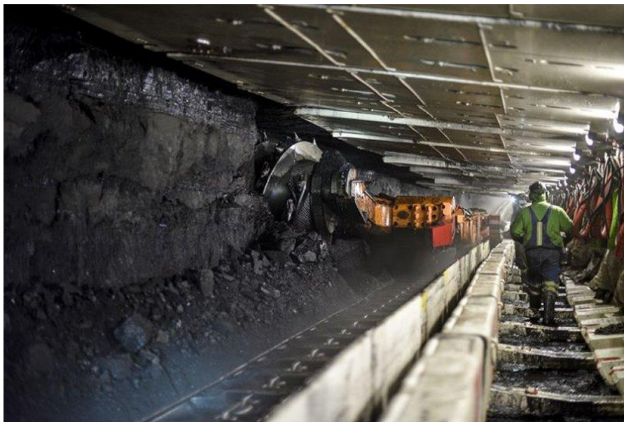
Longwall Mining at an Alabama Coal Mine, ca2020. (Alabama Mining Assn.)
