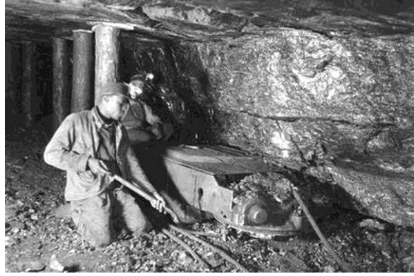
Mechanized coal cutting machines improved safety and productivity. (Library of Congress)
