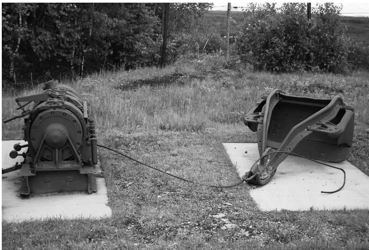
A Tugger-Scraper at Soudan Underground Mine State Park in Minnesota. The tugger unit is at left, with a modified hoe-type scraper at right. (Photograph by the author.)
