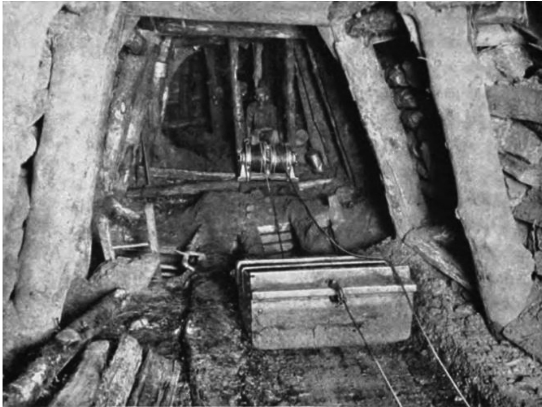
A double-drum scraper in action. The hoist engine is in the background. The scraper is pulling a load of ore toward a raise (covered with bars just in front of the scraper). Rope for power return is visible at the back of the scraper. (Charles E. Van Barnaveld, Mechanical Underground Loading in Metal Mines [Bulletin, University of Missouri School of Mines, Technical series, v. 7, no. 3] (Rolla, MO: U. S. Bureau of Mines and Missouri School of Mines and Metallurgy, 1924, 252.)
