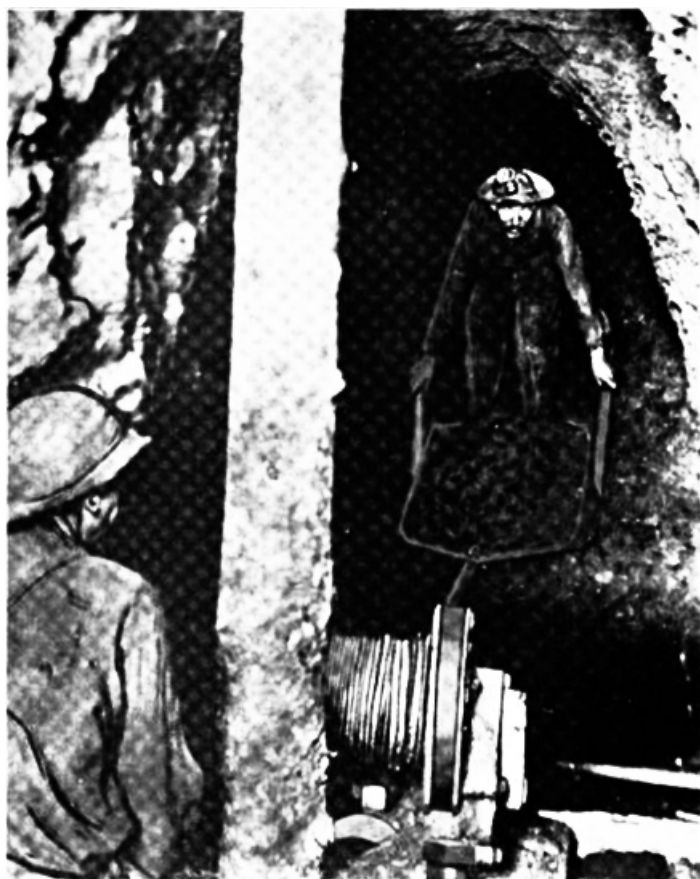
Slushing as initially applied by the Oliver Iron Mining Company, 1916-1920. A Uni-directional "Little Tugger" in the foreground, with a miner guiding a slip scraper in the background. The contents were dumped into the raise or chute in front of the tugger. The scraper required manual return to the mine face. (Lucien Eaton, "The Use of Scrapers in Metal Mines," Compressed Air, 26 (May 1921): 10067.)
