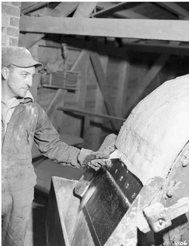
Workman tending a rotary filter at the Kramer Mill in 1942, by Ben Zellers. (Courtesy of the Western History Collection, Denver Public Library #6212.)
